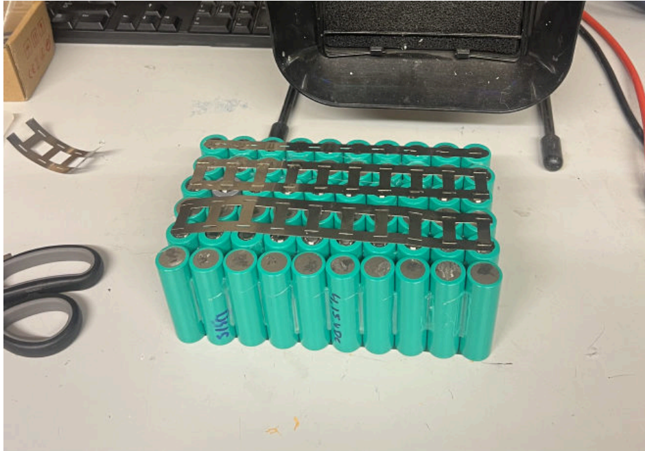
Figure 11: LIION-Battery during assembly
